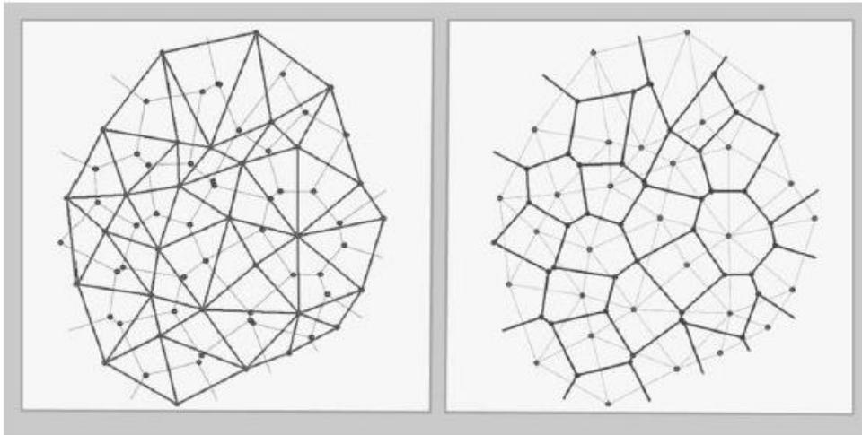
Fig. 1. Delaunay triangulation and Voronoi diagrams [5]
